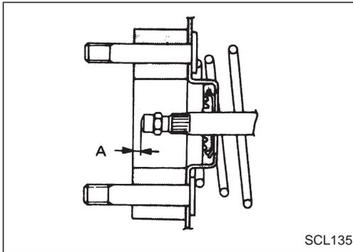
If amount of adjustment required exceeds 0.5 mm (0.020 in), reaction disc may have either been dislocated or fallen off. Replace clutch booster assembly.
