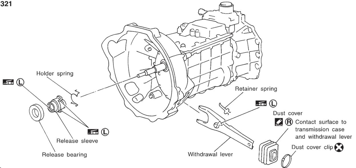
(L) : Apply lithium-based grease including molybdenum disulphide.
