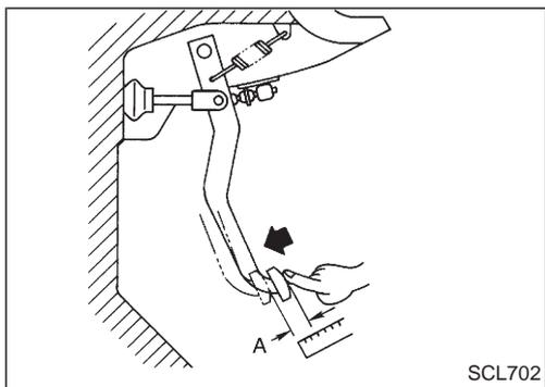
**Pedal free play means the following total measured at position of pedal pad:**
